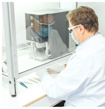
kind of setup are highly time-consuming and cost-intensive. However, they are an indispensable precondition for the reliability, independence, and validity of the analysis results. Even the unpacking of the samples and the SEM analyses themselves are conducted in a Class 5 cleanroom according to DIN EN ISO 14644-1 in order to prevent any sample contamination caused by the laboratory environment.
